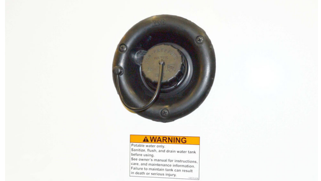
Water Tank Gravity Fill -Typical View
