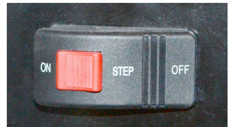
Entry Step Switch (Located near entrance door) -Typical View
